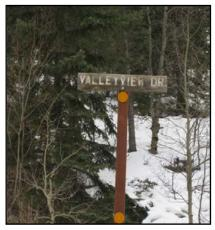
Figure 7. Combustible and difficult to read road sign.
