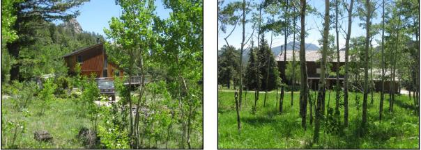
Figure 57. Typical homes in Porter Ranch/Twin Sisters area. Homes are lacking defensible space and many have combustible wood siding.
